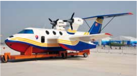
Reminiscent of Soviet-era ekranoplans, China's own wing-in-ground-effect craft, the HW-1
