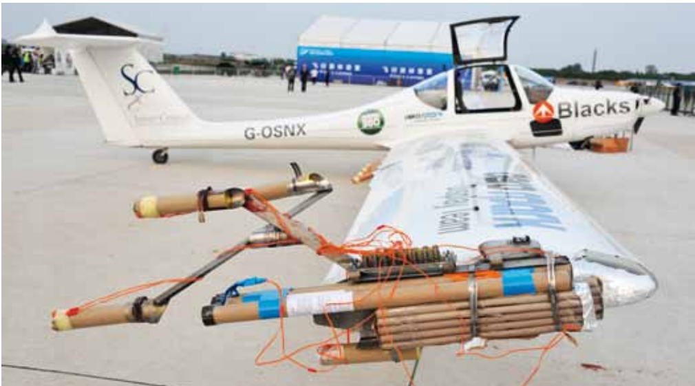
Taking the fireworks aloft: Chinese-made pyrotechnics mounted on one of the AeroSparx's Grob 109Bs
