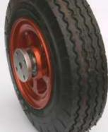
6" SL nose wheel for ultralight aircraft and LSA
