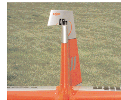
Just look at those control deflections, and those massive ailerons! The penalties for a flightpath a few degrees off vertical or 45° lines are horrendous, thus the wire sighting device on each wingtip (upper left photograph). Align the appropriate wire with the horizon, allow for wind, judges' position and you might get a high score.
