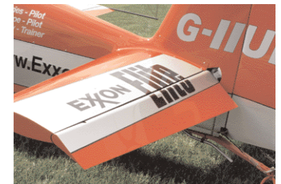
Just look at those control deflections, and those massive ailerons! The penalties for a flightpath a few degrees off vertical or 45° lines are horrendous, thus the wire sighting device on each wingtip (upper left photograph). Align the appropriate wire with the horizon, allow for wind, judges' position and you might get a high score.
