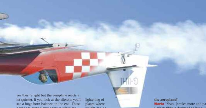
horns are quite clever because when the leading edge of the horn is centred it wants to stay in that neutral position. There's a lot of force needed to break out that long aileron but once it is deflected, the top surface of the horn balance is shaped like an aerofoil so helps to lift it out."
